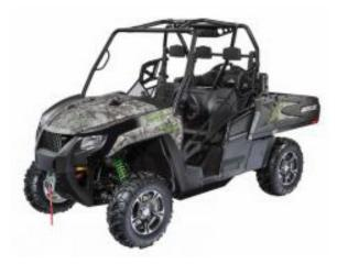
name is printed on the right and left front fender. The vehicle identification number (VIN) is located on the steel frame between the right front lower A-arm mounts. These vehicles were sold at Kawasaki dealers nationwide from July 2014 through June 2016 for between \$12,000 and \$16,900.
